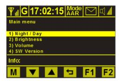
Press the scroll-down button once to scroll-down the menu bar to the sub-menu "Brightness":
