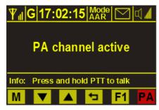
At the same time the PA start tone (see chapter 6.2.7) will be transmitted to the PA system as well as to the Clean Cab Radio loudspeaker.
