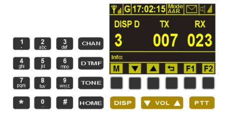
The numeric keypad, 0 through 9, # and \*, represents the traditional telephone-type keypad.
