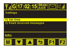
Press to select. The following input screen appears. The local time needs to be set in 24 hour format. Use the keypad to enter the time.
