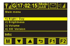
The sub menu "Night / Day" is highlighted. Press M again to enter. The display mode changes immediately to the other mode, in this case to the night design:
